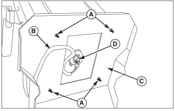
Figure 4. Remove The Existing Seat
